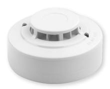
All of the Sentek's HD912 series detectors meet the requirements of UL521 and EN 54-5for use in fire alarm signaling systems, which provide fast and reliable response for heat 57°C (135°F) or Rate-of-Rise detection, They are intended for use in 2-wire/4-wire Class A2 supervised zone circuits. The HD912 series detectors are subject to panel compatibility limits and compliance with corresponding NFPA 72E standards, local codes, and ordinances.
